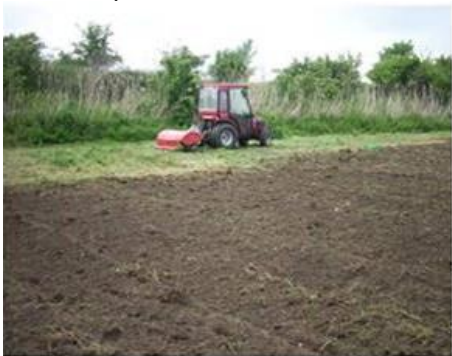
Figure 3: tilling by mill cutter
